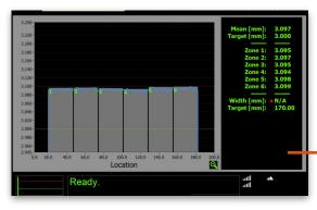
View thickness of sample in a range of zones
