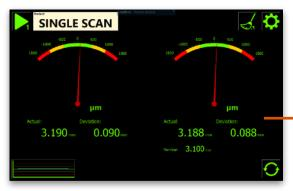
Needle gauge location showing left-right thickness
